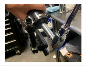
3. Use a chamferless socket to undo the TOPCAP.
