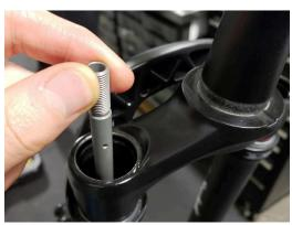
4. Thread a gear shift cable through the hole in the top of the INNER TUBE and through the new COIL SPRING. The COIL SPRING should be orientated with the HEAT SHRINK closest to the top.
