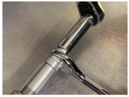
4. Using a 2mm hex key to keep the HBO NEEDLE from spinning, unthread the FOOTSTUD from the unit. Take care not to remove any shims which may stick to the FOOTSTUD when removing it. Shim Stack configuration as follows:
