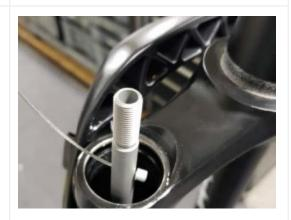
Use the shifter cable to pull the INNER TUBE up through the COIL SPRING until the threads of the INNER TUBE are exposed above the COIL SPRING.
