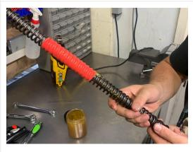
Install the SPRING ISOLATOR, it clips between the SPRING and the SPRING COLLAR in two pieces. Pull down on the spring to preload it and slide the SPRING ISOLATORS into place.
