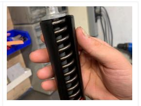
7. Thread the TOPCAP onto the INNER SHAFT ASSEMBLY.
