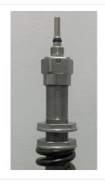
update April 2025: If your outer tube assembly came with two hex shaped preload collars, now continue to tighten the two collars against each other to lock them into place. You will need a 24mm cone wrench for one of them. Torque spec: 11.3 Nm or 100in/lbs
