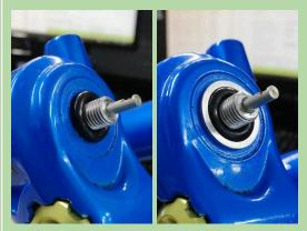
2. Use a Torque wrench and 12mm socket to torque the FOOTNUT to 55in.lbs (6.2Nm) without loctite.
