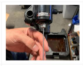
Using a 19mm Wrench to hold the BASE VALVE, Unthread the FOOTSTUD a quarter turn with an appropriately sized socket (size varies by footstud type).
