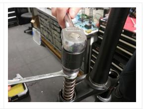
3. Remove SPRING COLLAR, SPRING ISOLATOR and COIL SPRING.
