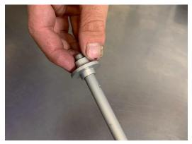
2. Install a stack height of TOP OUT SPRING SPACERS as required to suit your fork travel. TOP OUT SPRING SPACERS must sit on the INNER TUBE between TOP OUT SPRING ASSEMBLY and SEALHEAD. See table across for travel configurations. For example: a 180mm travel fork requires 20mm of TOP OUT SPRING SPACERS so install 1x 20mm spacer.
