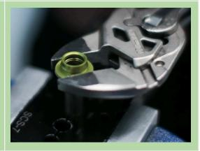
Stretch bottom out bumper over DAMPER side footstud, and onto the damper side shaft (in the same way that it was originally installed on the air side shaft). Ensure correct orientation – recess of bumper should seat around the footstud.
