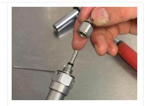
6. Using a 19mm wrench and an appropriately sized socket, torque the FOOTSTUD to 75 in.lbs (8.5N.m) without loctite.
