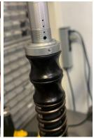
GENTLY snug the set screw against the flats on either side of the outer tube. DO NOT OVERTIGHTEN OR DAMAGE WILL OCCUR.
