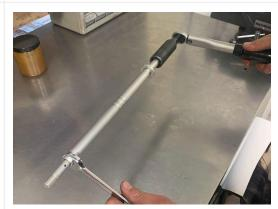
Position and install the included length of HEAT SHRINK just above the threads on the OUTER TUBE extending over the end of the SEAL HEAD using a heat gun.
