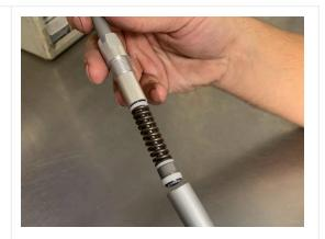
4. Using a 19mm deep socket on the BASE VALVE and 14mm wrench on the SEALHEAD torque to 75in.lbs (8.5Nm) without loctite.
